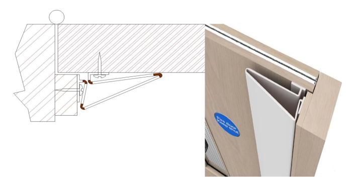
Digitex Front is a rigid / flexible PVC extruded safety strip which prevents fingers being jammed on the open hinge side of a door. When fitted the gap is covered completely and it is suitable for domestic or commercial use.
