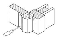
Line up the edge of the finger guard parallel to the guideline on the frame. Press firmly to hold in position before finally securing with the screws provided. For metal doors and kick plates pre drill with a 2.5mm drill bit.
