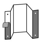
Remove one layer only of the double sided tape from each side of the finger guard device.
