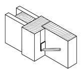
With the door in the closed position use a pencil / pen to draw a guideline on the door frame using the plastic measuring block (provided) in the vertical position (20mm)
