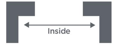
2. If required notch both ends of the Sill to allow it to fit into / around the Doorframe (as shown below) -
