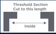
2. The clip-on-ramp is cut to the length across the internal rebate, it can be clipped into place prior to the installation of the threshold unit.
