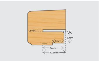
Automatically spaces the double glazed unit with a choice of 1mm to 6mm colour coded packer
